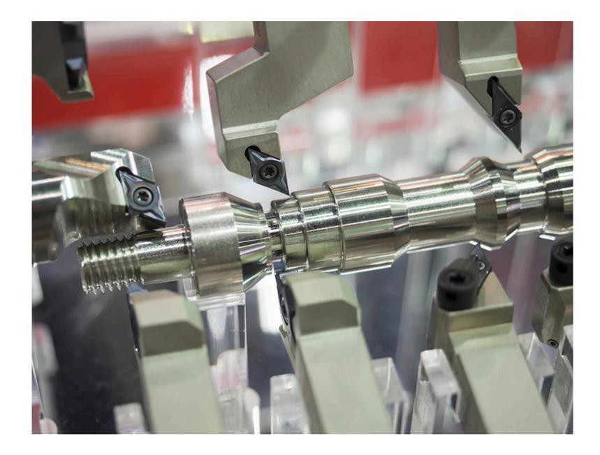
Operating both fixed and sliding head multi-axis turning centers, our machines accept materials up to 12 feet long, with diameters as small as .050" or as large as 3". Each machine has a sub spindle and features live tooling which allows us to make finished parts in one machine. We specialize in prCoduarcingt small or large quantities with a high volume rate due to our automated turning centers.
